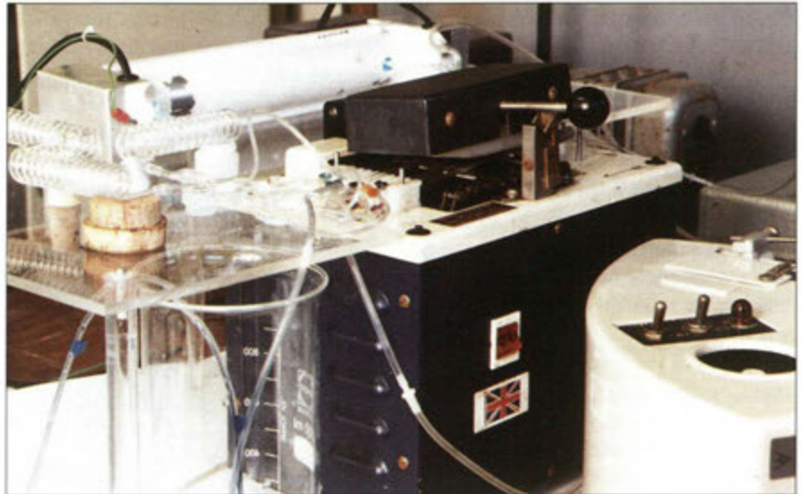
Figure 1. Equipment for measuring organic P in soil solutions.
