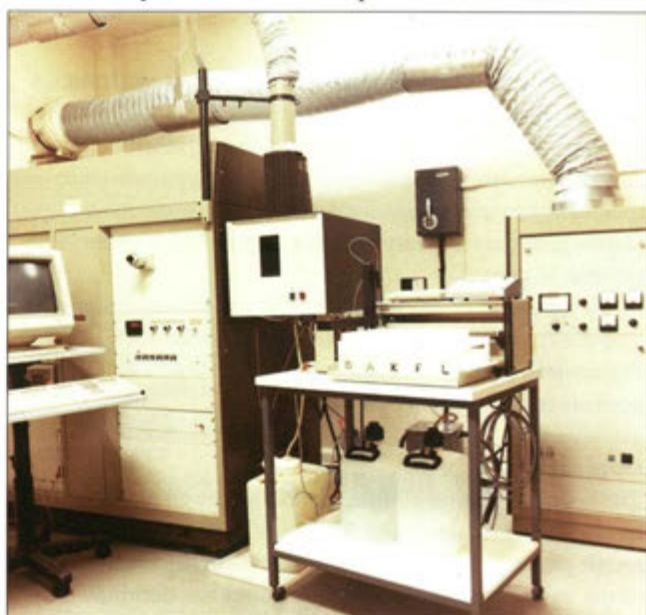
Figure 2. The concentration of a wide range of inorganic elements is estimated using Inductively Coupled Plasma Emission Spectrometry.
